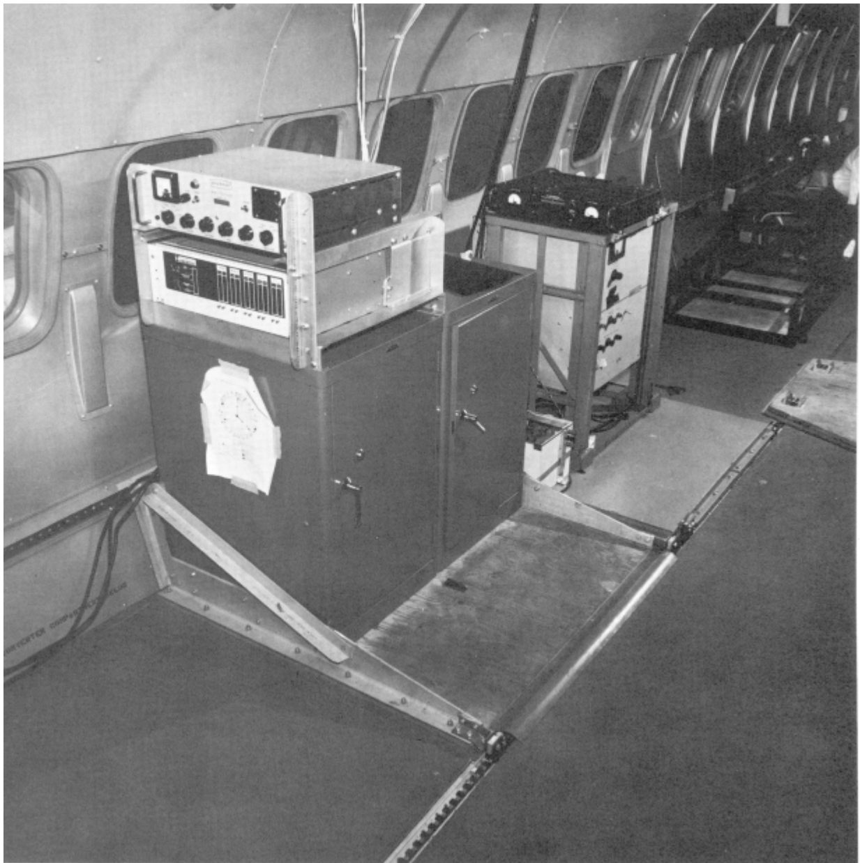
Figure 19.- Time code generator, WWV receiver, and auxiliary dc power supplies.
